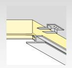
Attached directly to the ceiling or to suspended lattice with mounting brackets.
